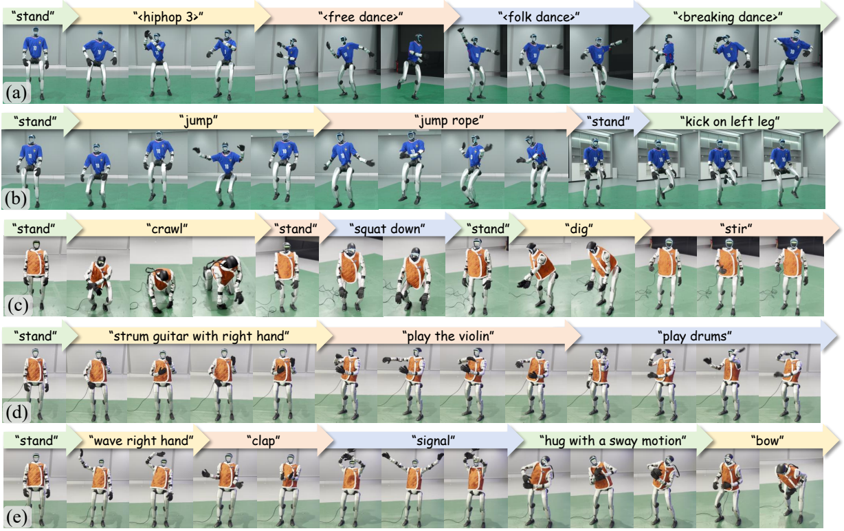
Fig. 4: Continuous diverse skill execution in the real robot. The robot seamlessly performs a wide range of tasks, including multiple dance styles, dynamic jumping behaviors, instrument-playing motions, and expressive gestures. For complex long-horizon motions in the private dataset, the entire motion is assigned a unique label wrapped with “<·>” markers.
